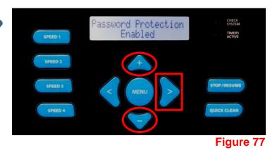
3. At this point (fig 79) you will be prompted to change the password by pressing the '+' button or skip by pressing the button.
